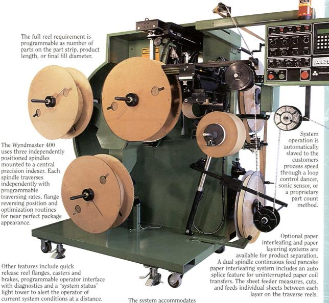
The system accommodates high speed stampings, rubber and plastic extrusions, and other product strips from any continuous process operations.
